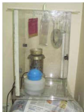
Fig. 5: A fuming chamber equipped with two heating systems
