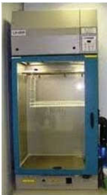
Fig. 1: A cyanoacrylate fuming chamber
